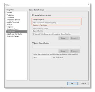
You can define up to three URLs. If multiple URLs are provided, the app will automatically distribute jobs across the specified Kongsberg Hubs, facilitating load balancing and improving overall performance. The Kongsberg Hub with the lowest total estimated production time is chosen.
